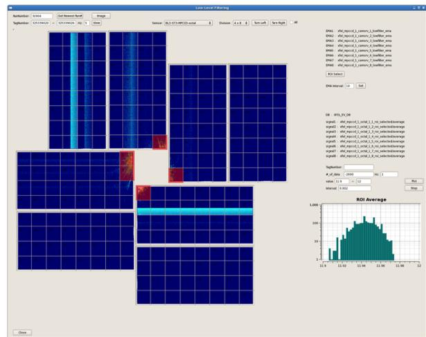
Figure 2: GUI image of the low-level filtering system. The region to the left shows MPCCD image data. A histogram of the ROI average photon number is shown in the lower right corner.
