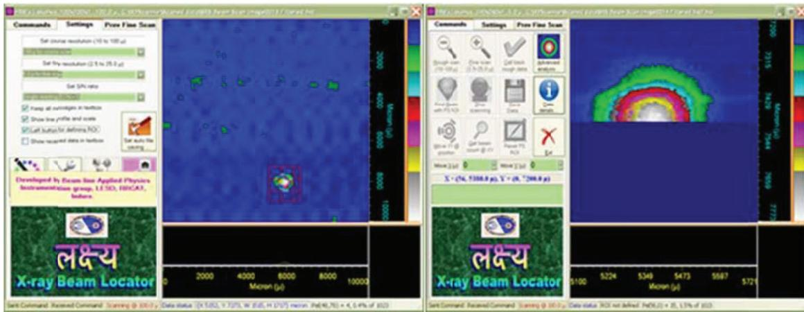
Figure 1: Main window of LAKSHYA shows marked rough scan image and fine scan in progress.
