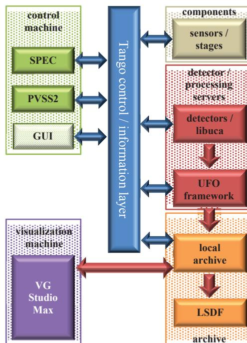
Figure 1: Communication (blue arrows) and dataflow (red arrows) between the different software layers and devices.
