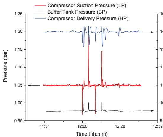
Figure 7: Buffer, LP and HP pressure curves at start and stop of a compressor with other two compressors running after implementation of the proposed control scheme.
