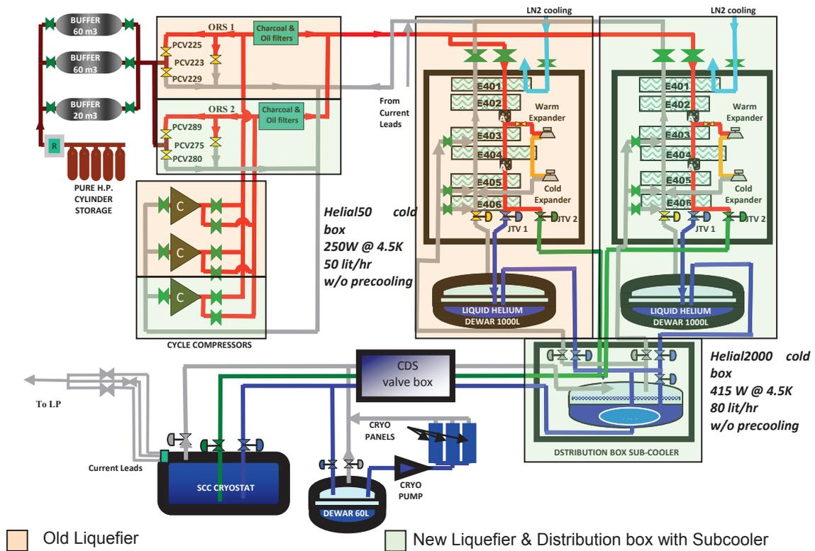
Figure 1: Schematic showing the cryogenic system consisting of buffer tanks, compressors, cold boxes, distribution boxes and cryogenic loads.
