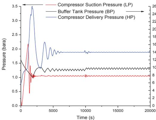
Figure 4: Simulation result (LP, HP and BP pressures) of warm helium process of the cryogenic system; with implementation of new unloading valve PID loop.
