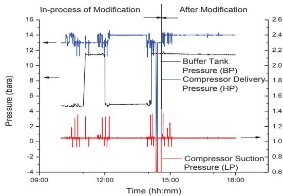
Figure 6: Buffer, LP and HP pressure curves before and after implementation of the proposed control scheme based on HP and buffer pressure.
