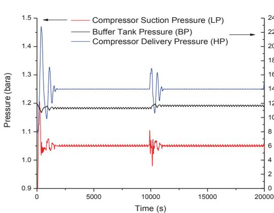
Figure 3: Simulation result (LP, HP and BP pressures) of warm helium process of the cryogenic system; only two normal PI loops are operational without any modification.
