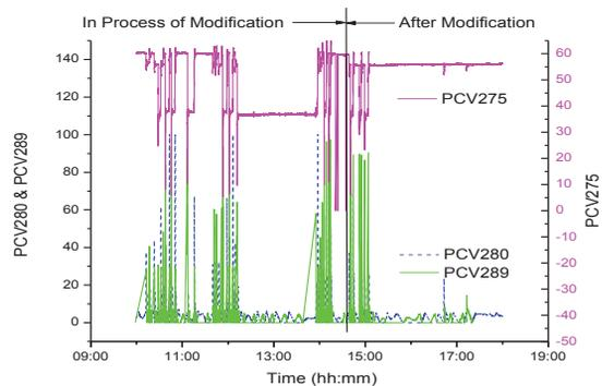
Figure 5: The fluctuation in opening of PCV289 to accommodate excess gas due to stopping of one compressor and that of PCV280 at the time of its start.
