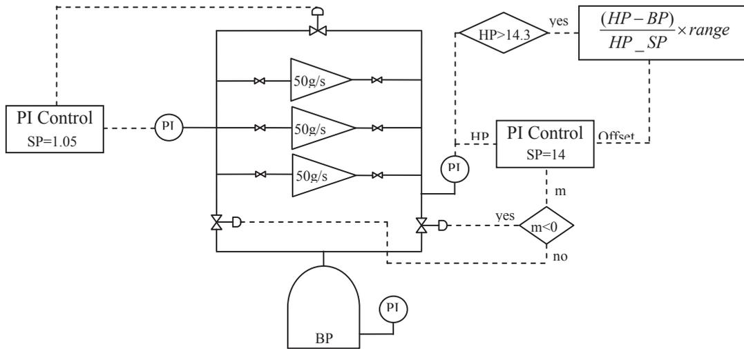
Figure 2: Pressure control of compressor suction and delivery for constant pressure operation of helium liquefier.
