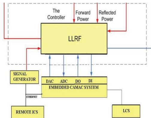
Figure 2: RF Control System – computer control.
