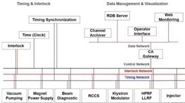
Figure 3: Block diagram of networked control system.
