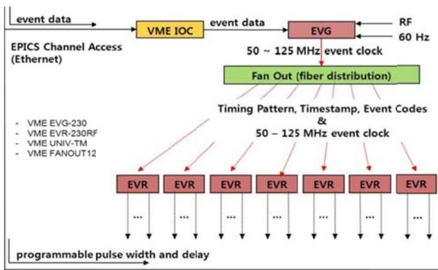
Figure 4: Architecture of upgraded timing system.
