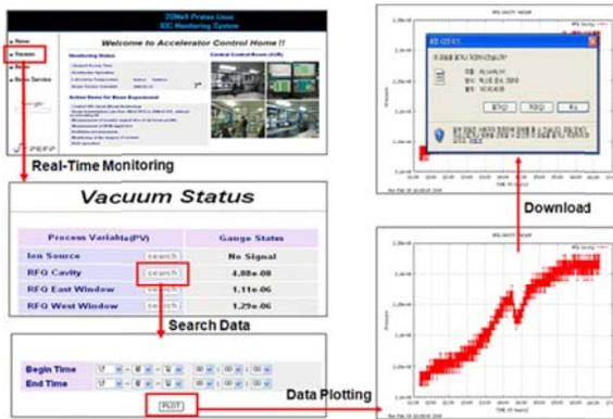
Figure 7: Web viewer for 20-MeV proton linac.
