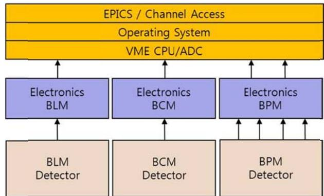
Figure 5: Schematics layout of EPICS system for beam monitoring.
