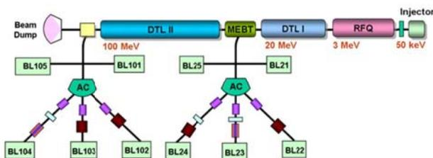
Figure 1: PEFP 100 MeV linac and extraction beam lines.
