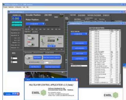
Figure 3. Multilayer monochromator GUI developed in Labview.
