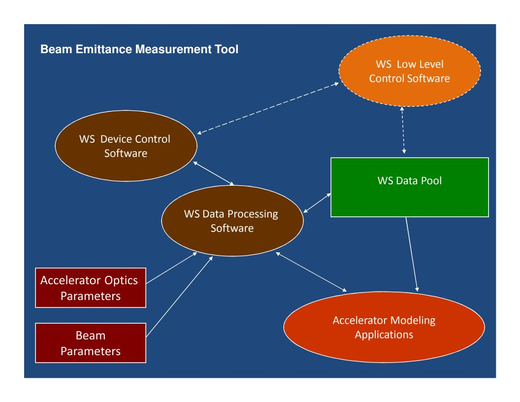
Beam Emittance Measurement Tool
