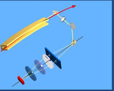
**Synchrotron Light Interferometer at location 1C12**
