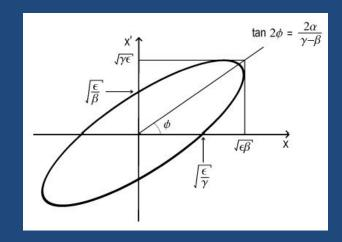
as a useful check, the beam-ellipse parameters should satisfy  $(\beta_x \gamma_x - 1) = \alpha^2$
