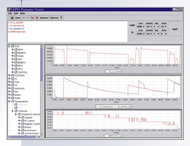
The handy graphical interface is developed for user's access parameters stored in the database. It provides observation of the stored data in graphical or textual form and monitoring of the values. parameter The interface allows us observe any collection of parameters in a single or in different diagrams (in subwindows) for any period of time. The interface provides the parameter's observation with varying time and amplitude resolution.
