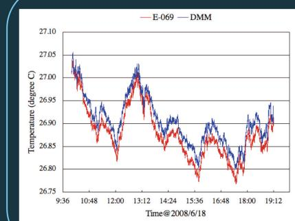
E-069 showed good results even during the accelerator operation and successfully realized almost the same measurement precision as the 6 1/2 digit DMM of about 0.01 degree C.
