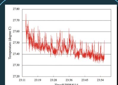
Measurement without connect the shield of the lead line to the analog ground of the module.
