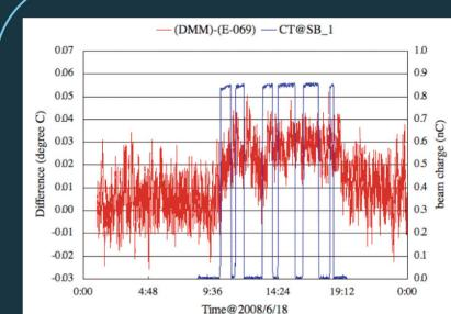
Difference between measured values obtained from E-069 and DMM.
