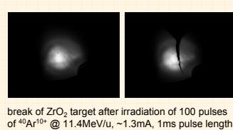
break of  $\text{ZrO}_2$  target after irradiation of 100 pulses of  $^{40}\text{Ar}^{15+}$  @ 11.4 MeV/u,  $\sim 1.3\text{mA}$ , 1ms pulse length,  $1.6 \times 10^{11}$  ppp
