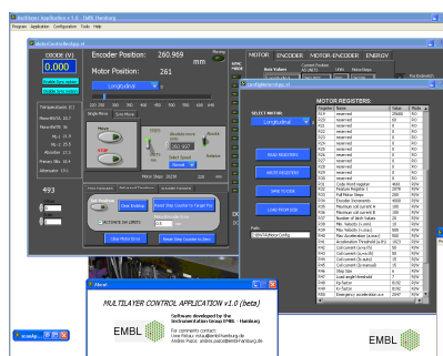
Figure 3. Multilayer monochromator GUI developed in Labview.
