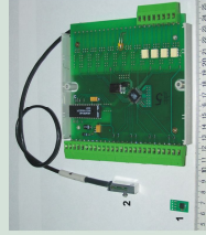
1 - sensor board; 2 - sensor inside the protection case
