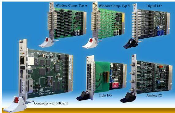
Figure 1: Interlock Controller and Slave Modules
