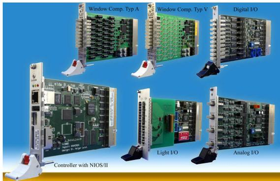
Figure 1: Interlock Controller and Slave Modules
