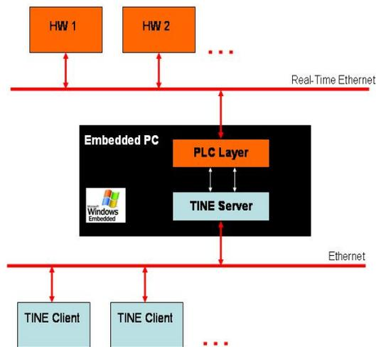
Figure 1: Distributed embedded design.
