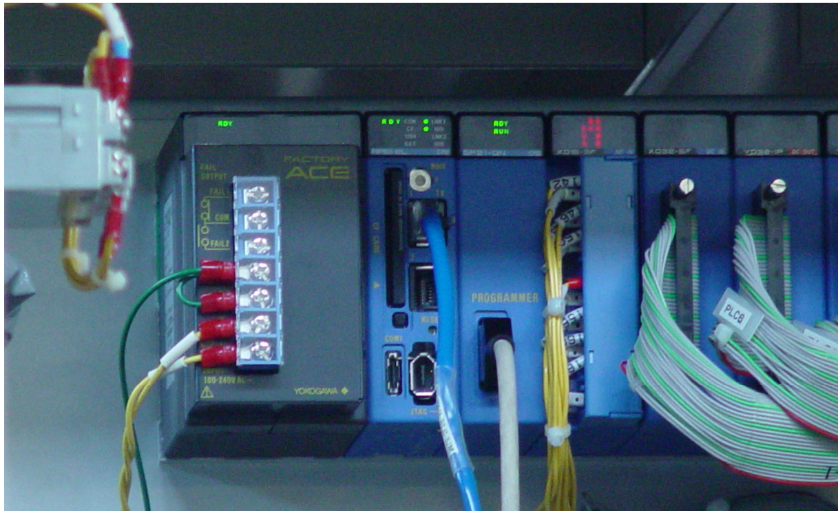
Figure 1: F3RP61-2L (the second left most module) serving as an EPICS IOC to control a septum magnet power supply for J-PARC Main Ring slow extraction
