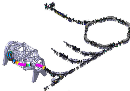
Figure 1: View of the facility: Two ion sources, LINAC, Synchrotron and four beam targets including the gantry.
