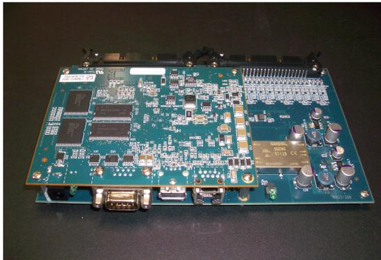
Figures 2: Pictures of E-069. The lower picture shows a CPU card (upper side) and a temperature measurement card (lower side).
