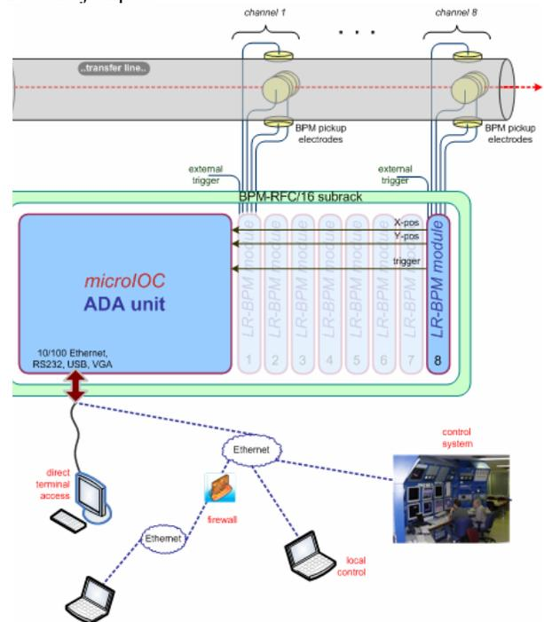
Figure 1: microIOC-LR-BPM schematic.
