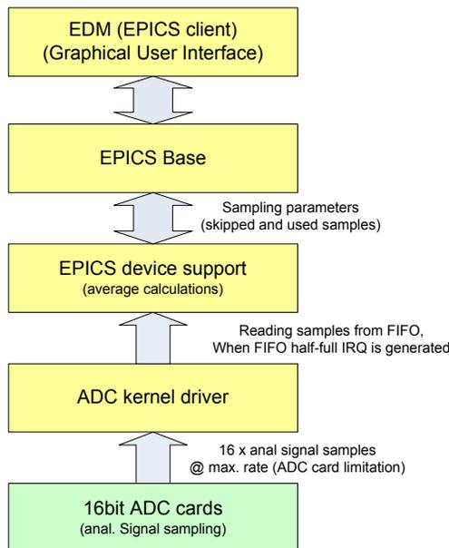
Figure 2: Software hierarchy of the microIOC-LR-BPM solution [2].
