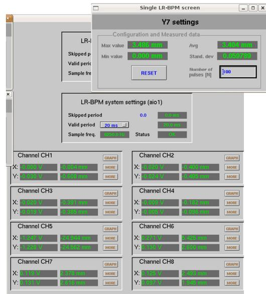
Figure 3: GUI application for 8 BPM systems. On the small screen in front user sees the minimum and the maximum value since the last reset. On the screen in the back user can set the Skipped and Valid period and values of the last bunch position (in V and mm) are displayed.
