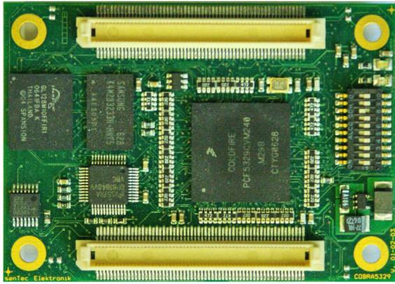
Figure 2: Picture of COBRA5329 board.
