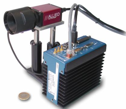
Figure 1: National Instruments Compact Vision System 1456 [2] with attached FireWire camera and remote controlled iris lens system.
