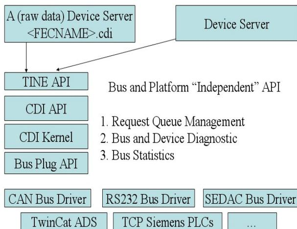
Figure 1: Architecture of the Common Device Interface
