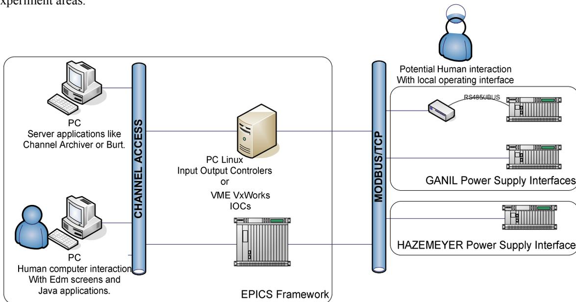
Figure 2: PC architecture schema of the power supply command control
