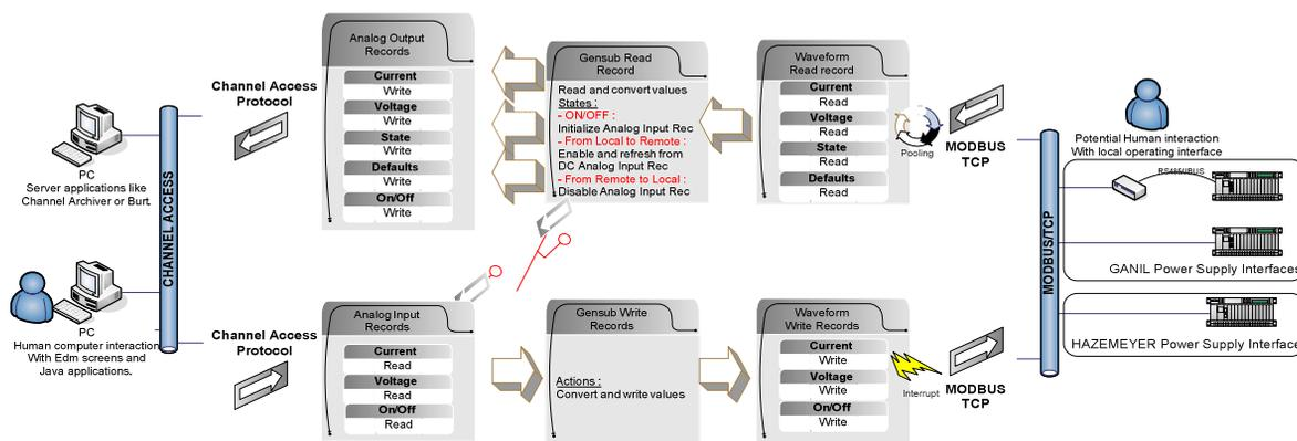
Figure 3: Data flow schema of the EPICS IOC database.
