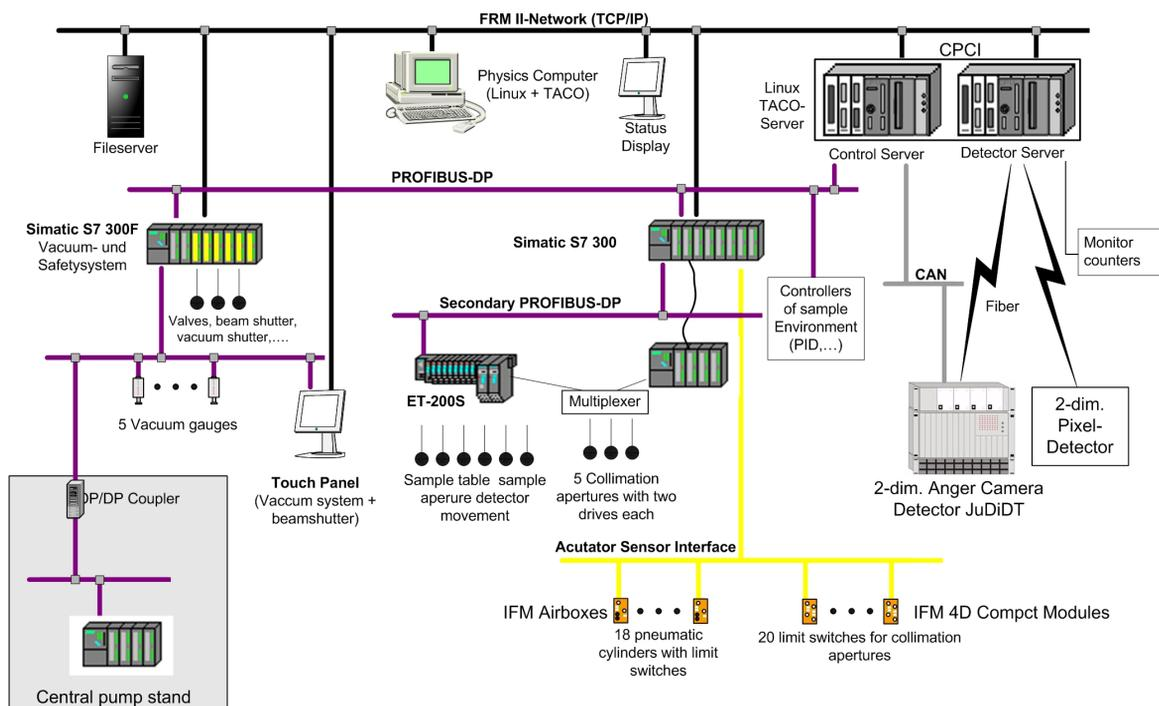
Figure 1: Physical structure of the control and data acquisition system of KWS2.
