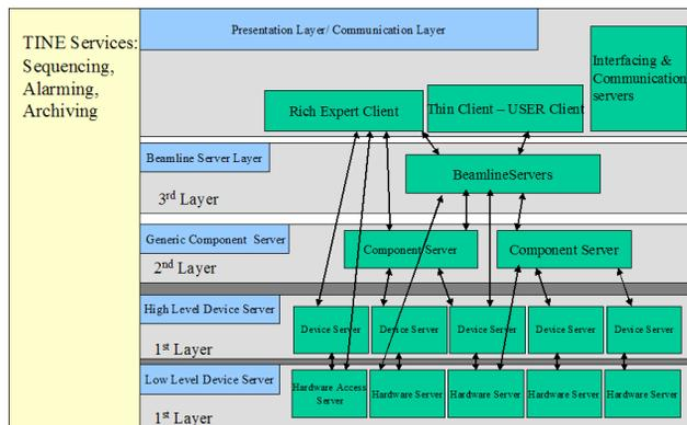
Figure 2: Beam line control layer concept
