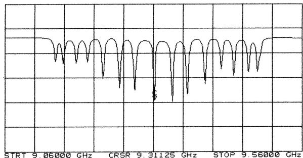
Fig. 6 Modules of Complex Reflection vs. Frequency
