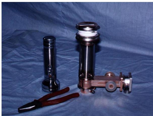
Fig. 8. 2 MeV On-axis SW Guide Braze Assembly
