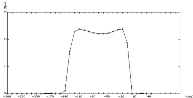
Fig. 4. Energy Spectra as a Function of Input Phase
