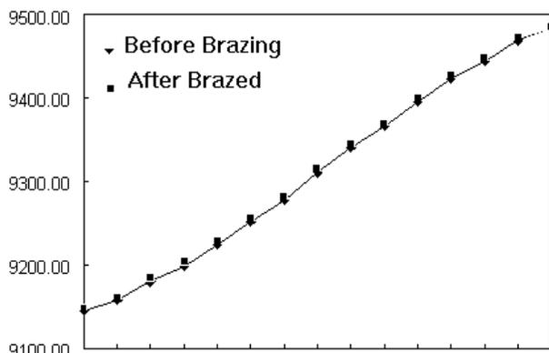
Fig. 7 Dispersion Curve for On-axis Coupled SW Accelerator Structure
