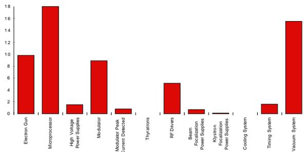
Figure 2: Linac subsystems downtime statistics (run 28-38) in percentage of the total machine downtime.
