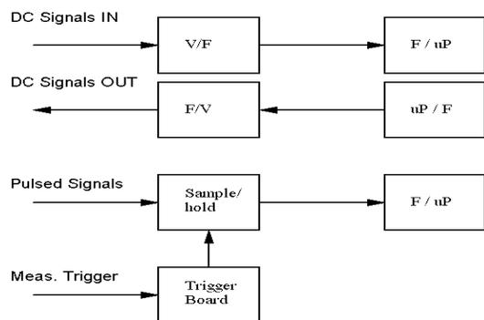
Figure 4: Layout of the analog signals acquisition scheme with voltage/frequency converters.
