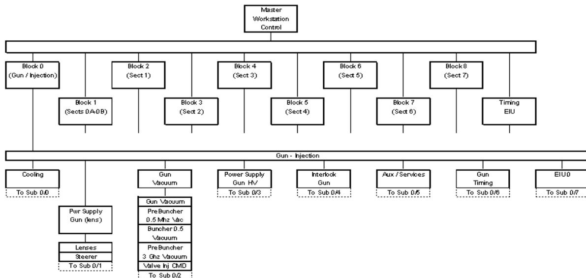
Figure 3 Block diagram of the new machine control system with an exploded view of the block 0.
