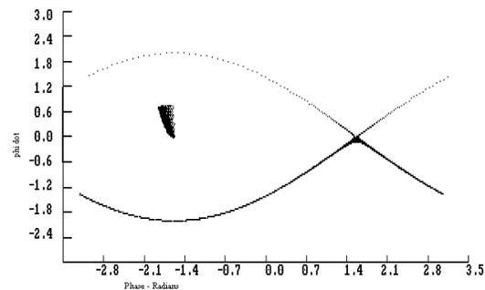
Figure 1 Phase of Extraction for Various Amplitudes of Synchrotron Oscillations.
