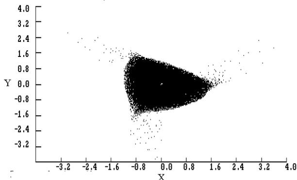
Figure 2 Extraction Separatrixes, RF Dipole Off
