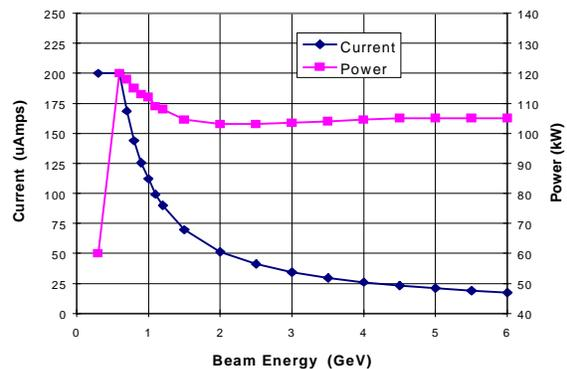
FIGURE 1. Current and power ratings for the commissioning and tune-up dumps.
