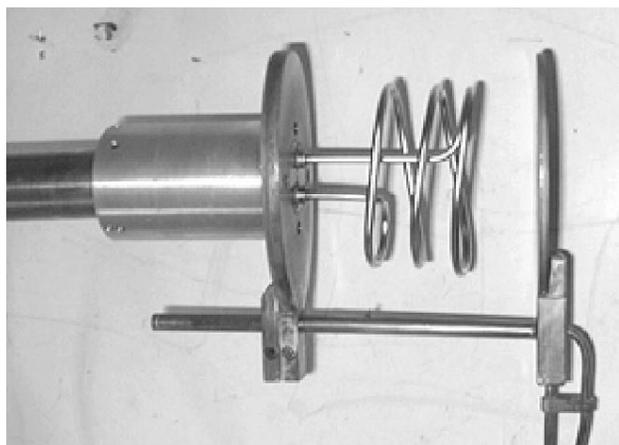
Fig. 2 A picture showing the water-cooled titanium rf induction antenna.
