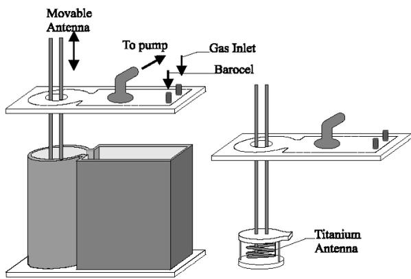
Fig. 1 Experimental setup for TiN coating of a B-factory beamline chamber
