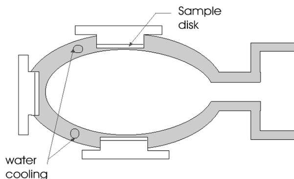
Fig. 3 A schematic diagram showing the locations of the three sample disks when they are mounted in the beamline chamber.
