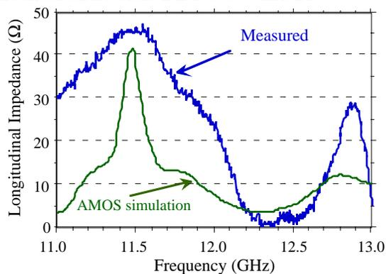
Figure 4. Comparison of measurement and simulation for a solid rexolite insulator.
