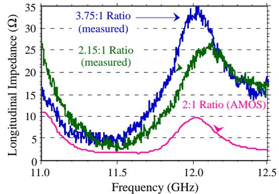
Figure 5. Comparison of ratios of insulator to conductor thickness in the stacked insulator. Decreased effective gap width generally reduced resonant peaks with minimal effect on the “valleys” between peaks.
