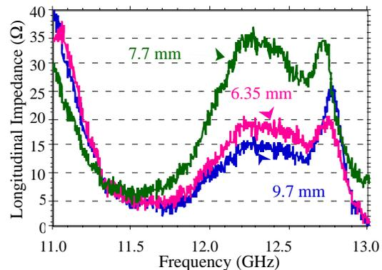
Figure 3. Effect of different gap widths on  $Z_L$ . Above the cutoff frequency, peak impedances did not obey the linear scaling with gap width predicted by analytical theory.
