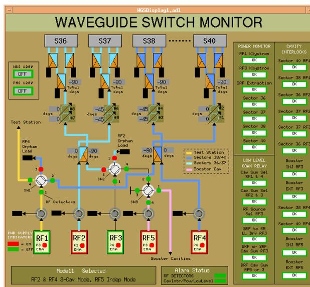
Figure 1: The APS rf system switching control screen.
