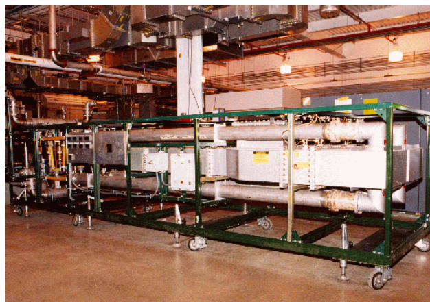
Figure 1: Side view of the rf load.
