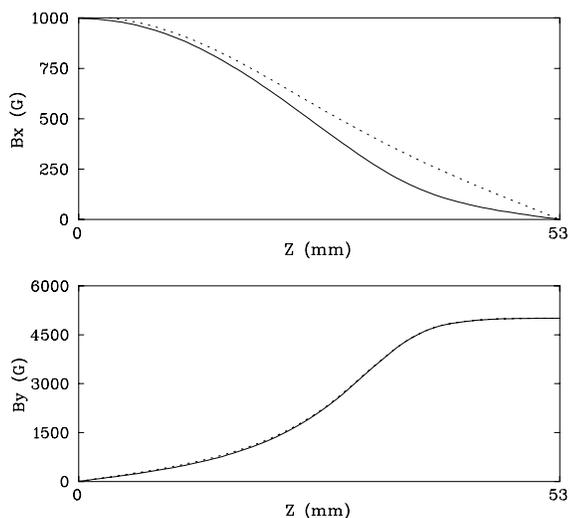
Figure 2. Field distributions in the final EEW design (solid lines) and in the case with only poles of a single type present (dotted lines).
