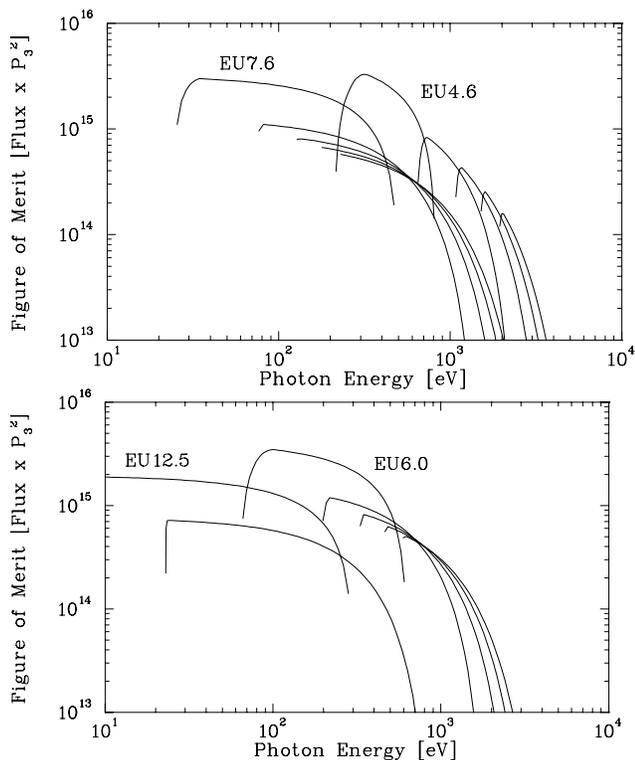
Figure 2. Performance of the proposed elliptical undulators in the circular polarization mode (2 GeV, 0.4 A).
