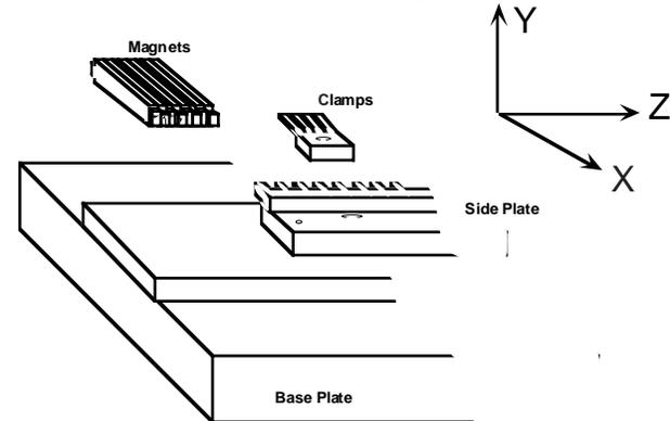
Figure 1. Magnet and holder structures
