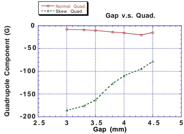
Figure 3-(b). Gap versus quadrupole components of the field.
