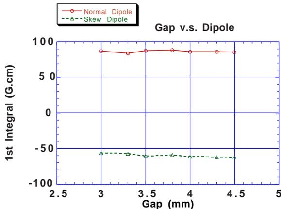
Figure 3-(a). Gap versus dipole components of the field
