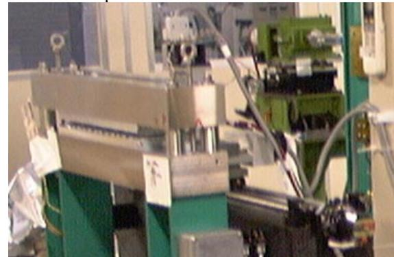
Figure 2. Hall probe field mapping system and rotating coil system.
