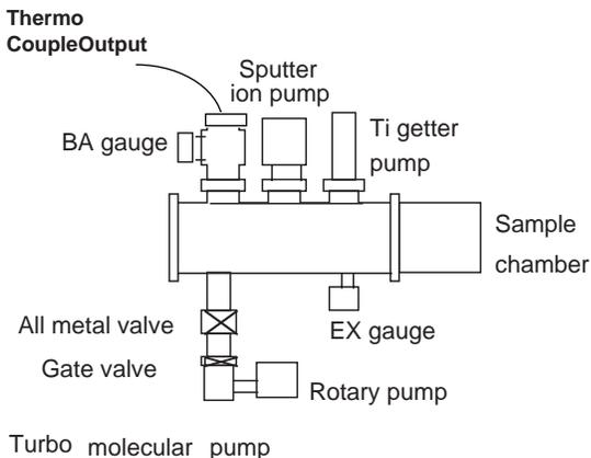
Figure 6. Schematic of the vacuum testing facility
