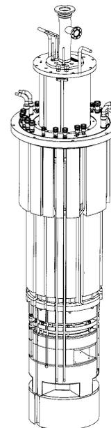
Figure: 1 The TMRS insert. The proton beam enters vertically through the pipe at the top. The openings for the neutron flight paths can be seen near the bottom.
