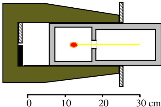
Fig 2. Dipole yoke, 4 conductors and vacuum chamber
