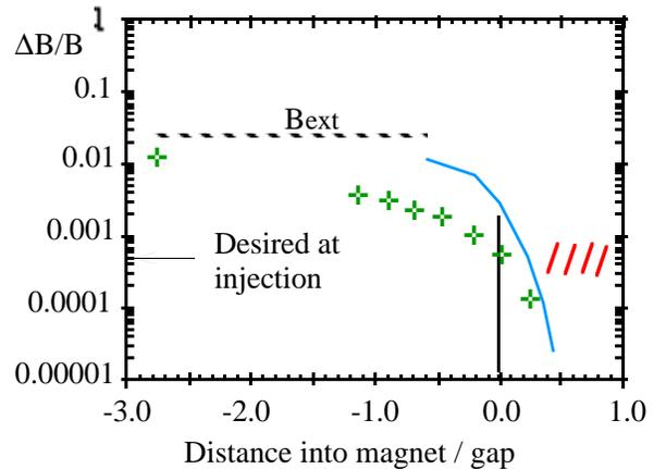
Figure 2, Measured error fields after degaussing, with parametrizations of Brown and Spencer.  $\Delta B/B = (\text{measured field}) / (\text{field at injection})$ , which is equivalent to the measured field in mT. The hatched line shows level of residual fields.
