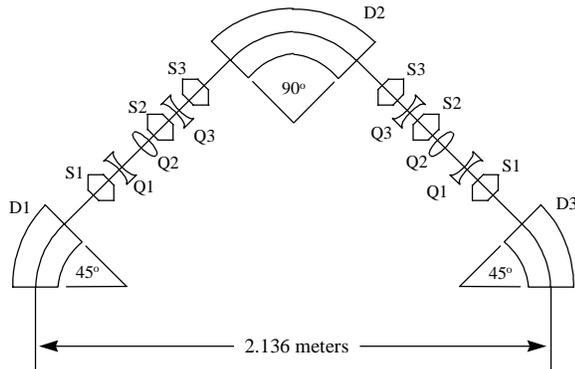
Figure 1. The isochronous 180 degree Dundee bend used to compute CSR emittance growth and emittance compensation.
