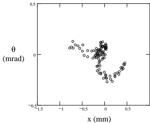
Figure 5. Transverse phase space at the exit of the bend for a S2 sextupole tip field of 4 KG.
