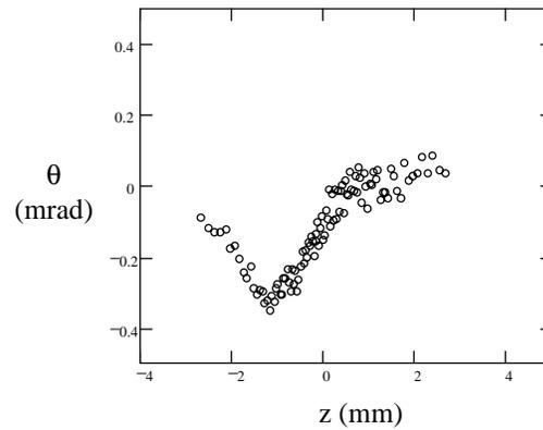
Figure 3. The correlation between beam divergence and longitudinal position in the microbunch for sextupoles  $S2_{tip} = 0$  KG.
