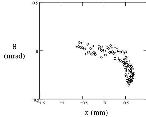
Figure 2. The transverse phase space at the exit of the Dundee bend for sextupoles  $S2_{tip} = 0$  KG.
