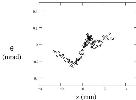
Figure 6. The correlation between beam divergence and longitudinal position in the microbunch for S2 at 4 KG.
