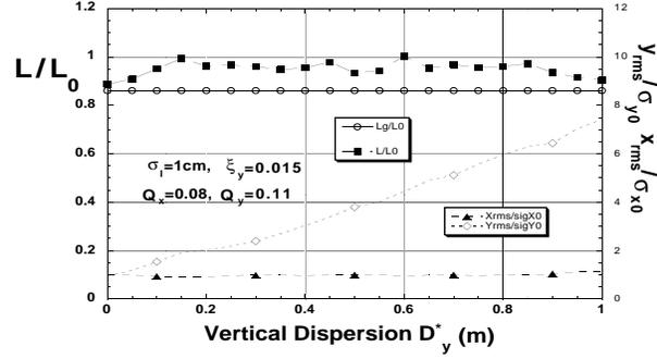
Figure 6: Luminosity and beam size vs.  $D_y^*$ .
