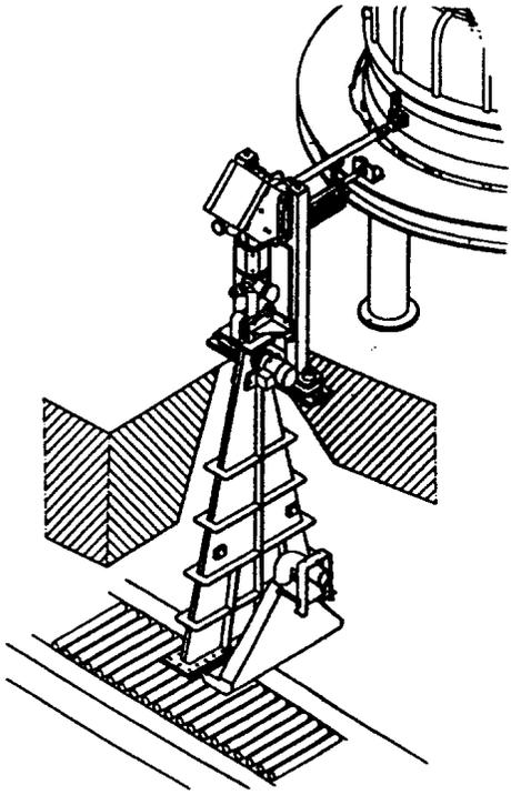
Figure 1: schematic of the standard beam delivery system for Rhodotrons
