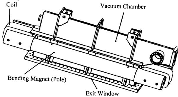
Figure 3 : mechanical drawing of the non-diverging scan horn
