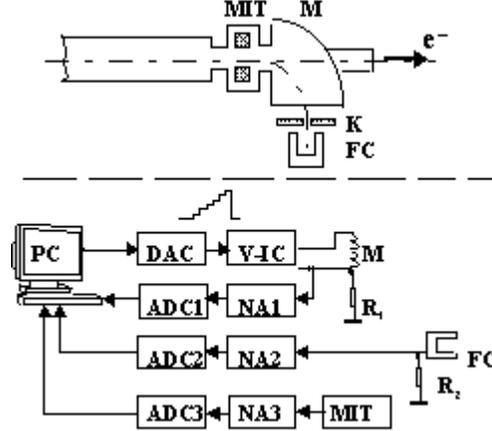
Fig. 1. Magnetic analyzer schematic
