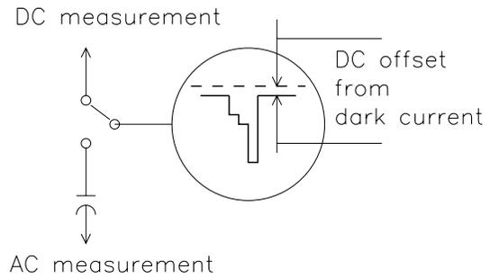
Figure 2: The essential difference between the AC and DC method is the capacitor which removes the dark current d.c. component in the AC method.
