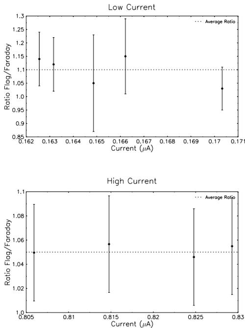
Figure 4: These two figures show the comparison between the flag and Faraday cup measurements using high current and low current conditions with the DC method. The flag intercepts more charge than the Faraday cup because the flag is upstream w.r.t. Faraday cup.
