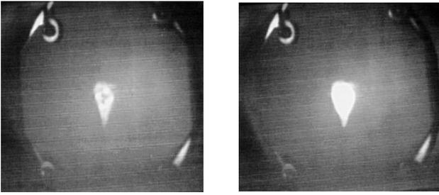
Figure 3: These photographs show how the structure of the dark current sources evolves through time. These photographs were taken 5 hours apart with the earlier photograph the left. Clear structural changes took place during the intervening period. These structural changes come from cycling the beam on and off during the 5 hours.
