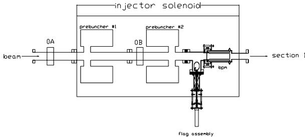
Figure 1: This is the overall layout of the injector. There are steerings in both the vertical and horizontal direction. By varying the phase and field strength of prebuncher 1 and 2, the amount of bunching and acceleration of the beam can be changed.
