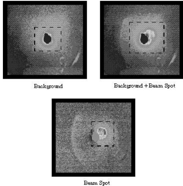
Figure 6: We show the process of digitization and image manipulation here: (i) background image is taken with the dark current, (ii) an image with both the dark current and the beam is taken, (iii) finally an image difference reveal the beam spot.
