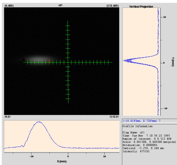
Figure 3: Beam on UF1. Scale ticks are in mm.
