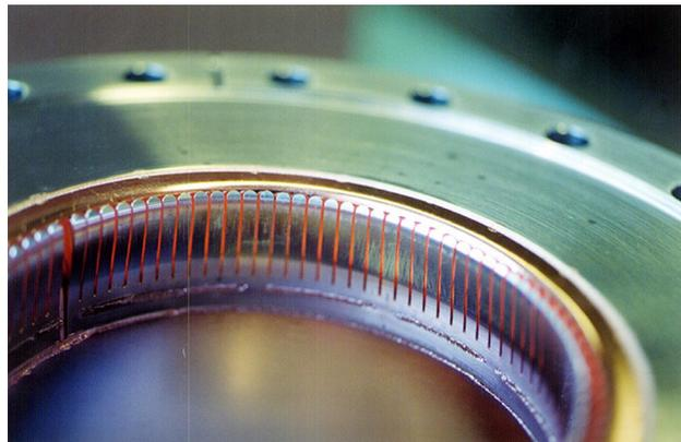
Figure 4. Spring Fingers as welded into Mounting
