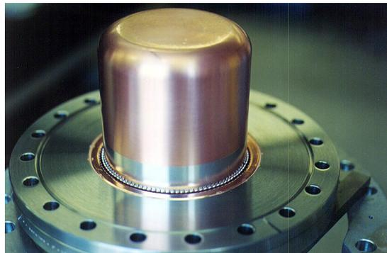
Figure 1: Tuner Assembly showing Plunger and Mounting Flange with Spring Fingers.
