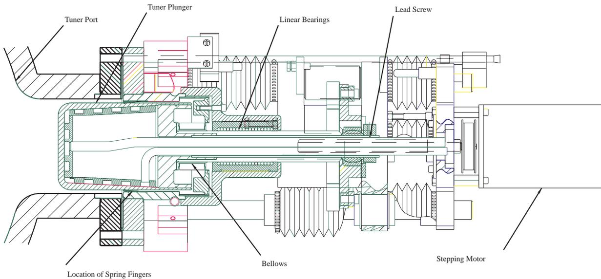
Figure 2. Tuner Cross-Section with Stepping Motor Drive.
