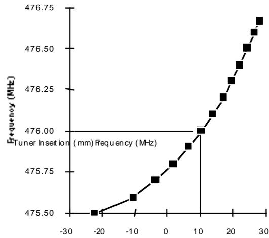
Figure 6. Cavity frequency versus tuner insertion.
