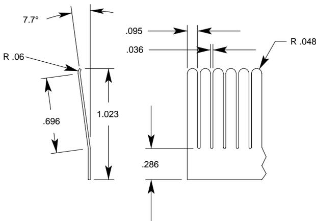
Figure 3. Spring finger Dimensions in Inches.
