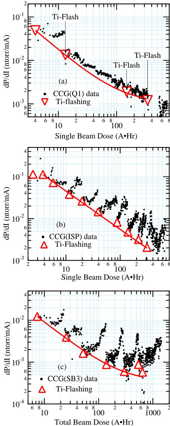
**Figure 3.** The beam induced dynamic pressure rise, ( $dP/dI$ ), at various locations in the IR. (a) At Q1E chamber; (b) on the beamline next to the ISP chambers, and (c) for the soft-bend chambers. (d) shows  $dP/dI$  for a gauge within the hard-bend sector pumped only by distributed ion pumps, where the SR flux and gas load are the most intense.
