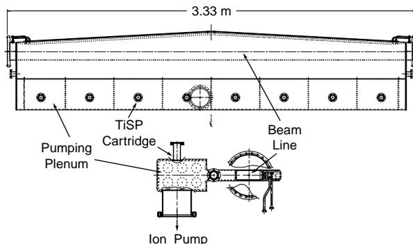
Figure 2. The Soft-Bend Chamber. Top view (above) and cross-section showing Ti pumping plenum.
