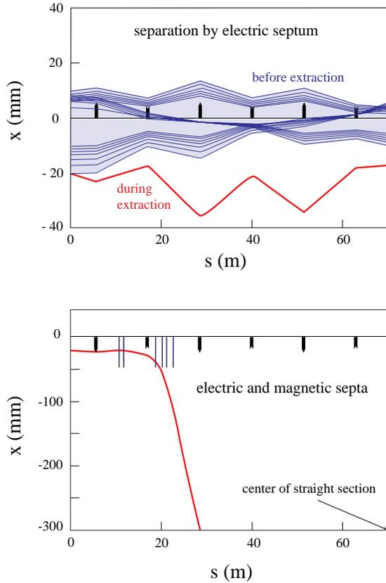
Figure 4: Extraction channel
