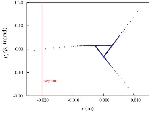
Figure 2: Separatrix triangle (with ELFE@DESY parameters)
