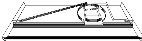
Figure 2: MAFIA 3-d model for the dipole chamber with a 15 mm wide slot for synchrotron radiation and a radiation absorber suspended in a cylindrical pumping port.
