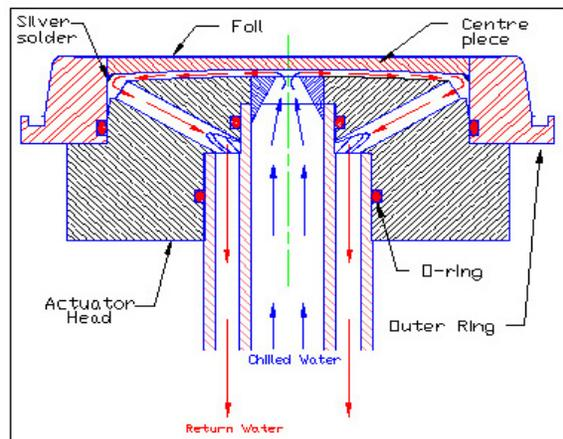
Figure 2: Target and Actuator Head cross section
