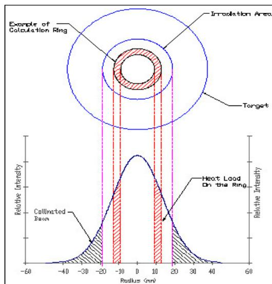
Figure 3: Proton Beam Power Density Curve
