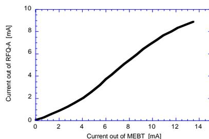
Figure 4. Beam current from RFQ-A as a function of beam current from MEBT at 30 Hz.
